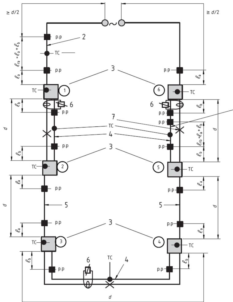
If the difference between the main and branch electrical cross-sections is greater than half a step as defined below, this test loop shall be used.
