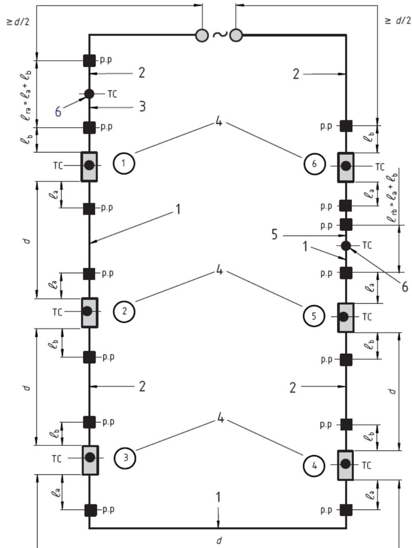
When the connectors have equal cross-section, then  $l_a = l_b$  and  $l_{ra} = l_{rb}$
